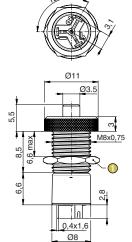
1 nut: 10 across flats, max tightening torque 1 N.m
