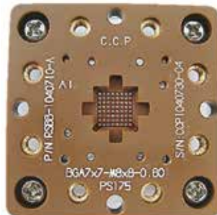
BGA Socket Pitch 0.8mm
